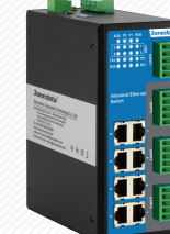
IES618-4D Series 8-port 100M + 4 serial ports
